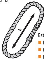
Estrope  $\varnothing$  14 mm
